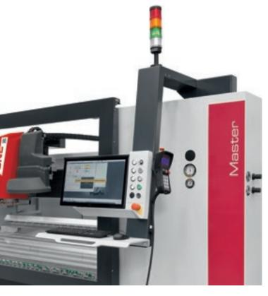
Built-in control panel, with optional touch screen, on the left side of the machine, with the option of installing it on the right side as well.
