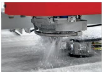
**External water pressure intensifier for perfect regulation** A circular wheel with small nozzles increases the pressure of external water. The optional device has a 3-position vertical movement to ensure that the water impact point is always the best, regardless of tool radius and height. Ideal for machining with grinding wheels and for kitchen tops.
