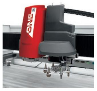
**Tool change in 10 second** The fastest solution in the world of stone, thanks to the 8-position revolver magazine on the head (6 positions with C axis).
