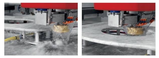
Grinding and polishing of bathroom unit tops: internal and external hole polished.
