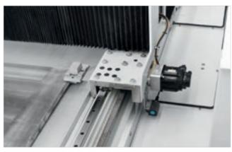
Rack and pinion for movement along the X and Y axis with more than twice the speed and acceleration. The helical teeth on the racks guarantee ultimate reliability.
