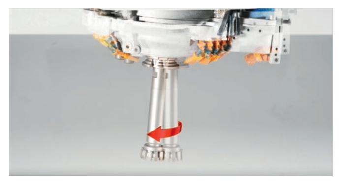
SINGLE DIRECTION TILTING T AXIS TO CREATE INCLINED RECESSES FOR KITCHEN TOPS.
