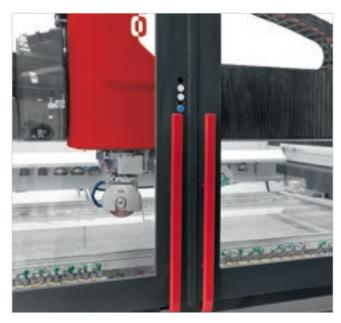
Electric safety lock with an ergonomic built-in button panel for opening doors and starting the machining operation, offering ultimate speed and comfort for the operator.
