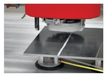
**3-axis head mechanical thickness tracer** The variable Z thickness tracer maintains a constant machining quality even on pieces with an irregular thickness.
